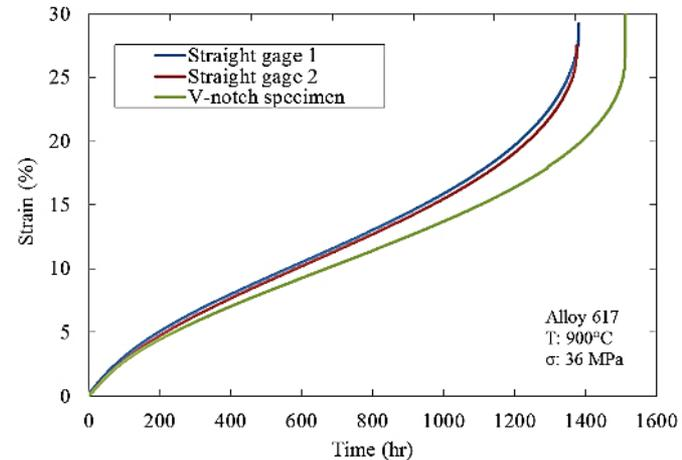
Creep results for V-notch specimens with extensometers over the straight gauge section and tested at 750, 800, and 900°C.
