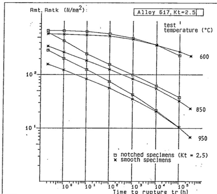
Isothermal stress-rupture curves for notched and smooth 617 specimens (notch radius 0.5 mm)
