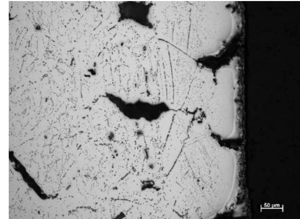
Optical micrographs after electrochemical etch showing cracking occurring at the grain boundaries for both (left) the 800°C and (right) the 900°C tests.
