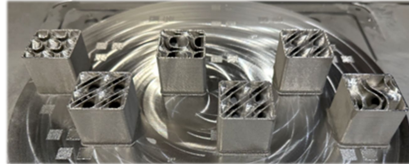
Sample Cladding Lattices Produced by Specialized L-PBF Process (StarHagen company)
