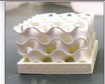
U-10Zr pellet fabricated by LENS technique
