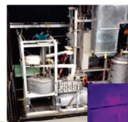
ORNL Liquid Salt Test Loop – configuration and thermal image
