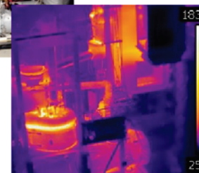
ORNL Liquid Salt Test Loop – configuration and thermal image
