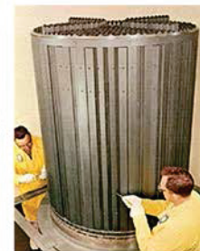
MSRE core - graphite - 69 ft 3 - 513 core blocks
