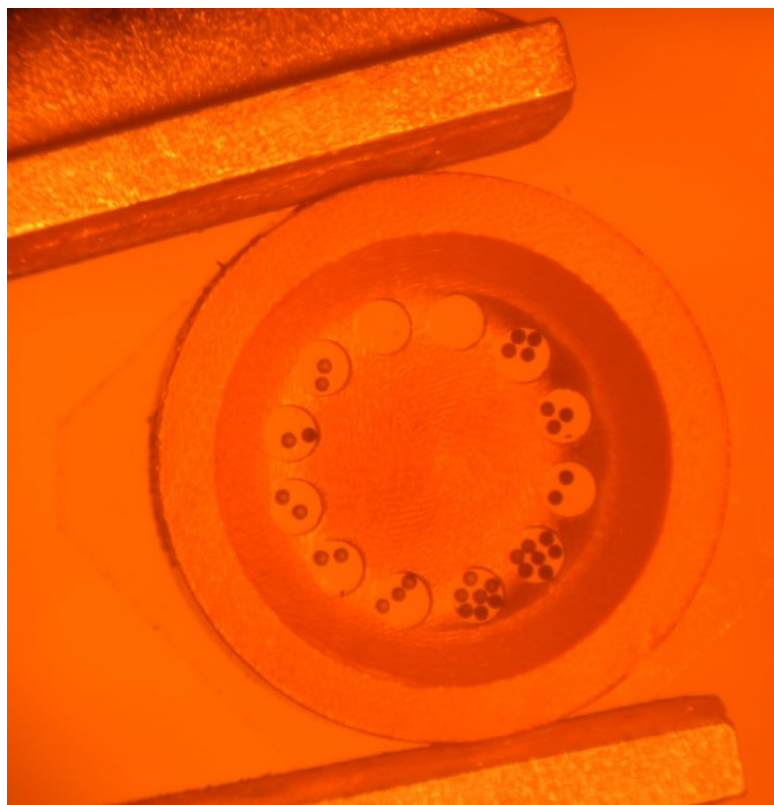
Figure 7. Mount with particles in the wells, adhered to Wafermount at the bottom of the wells, prior to addition of epoxy.
