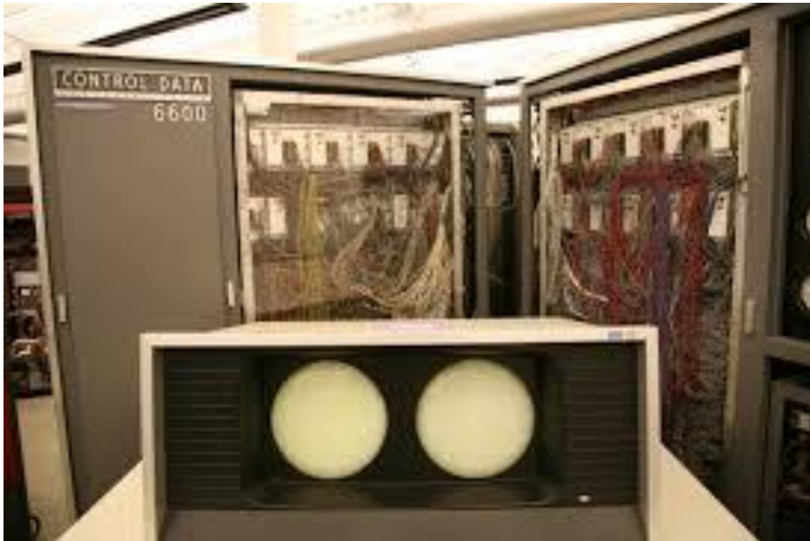
The CDC 6600: The "First" Supercomputer (1964) Peak performance: 1 Megaflops
