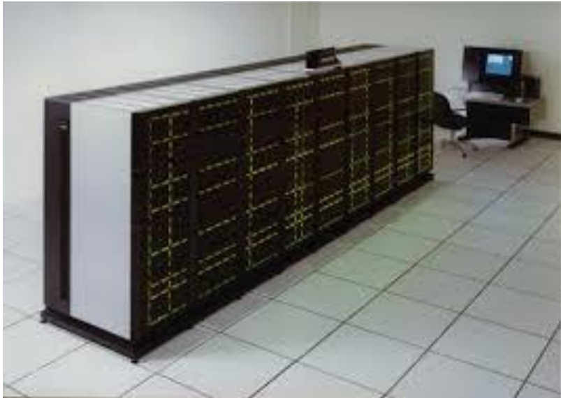
Touchstone Delta (1990s). 500 cores connected by mesh topology. 10-20 Gigafllops.
