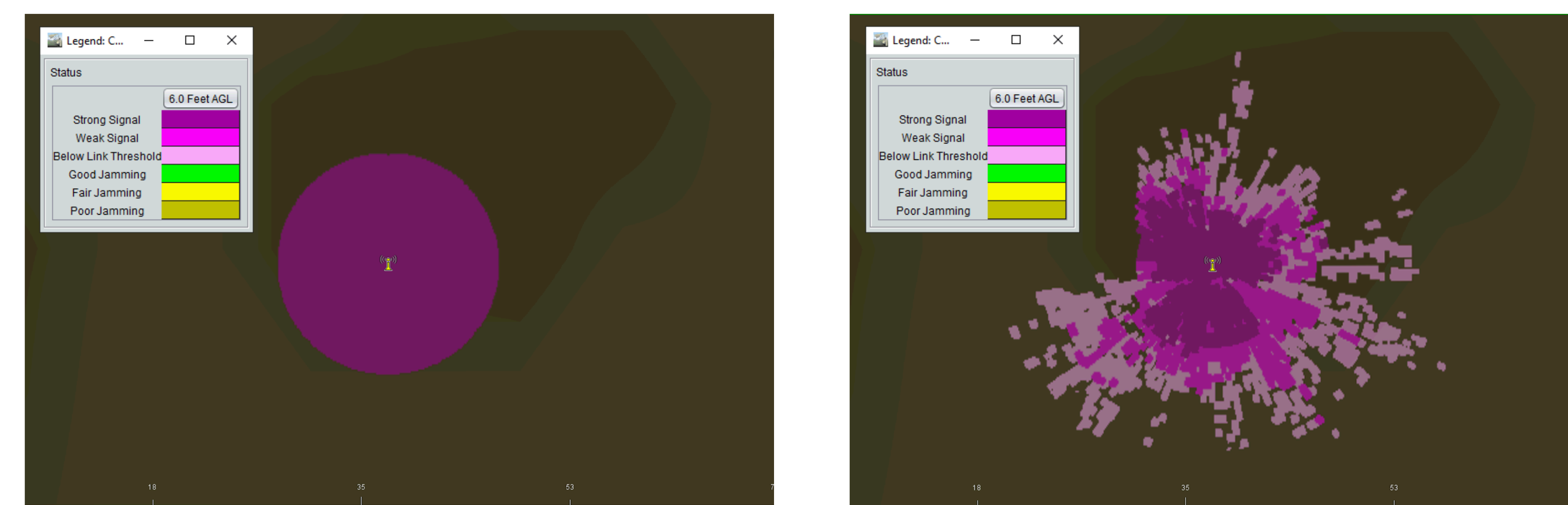
Figure 4. EWMSS' modeling capabilities: Collection Coverage Analysis results for WComm UCC Enhanced Model 210-C. Free space propagation, terrain not used in analysis (left). TIREM propagation, terrain used in analysis.
