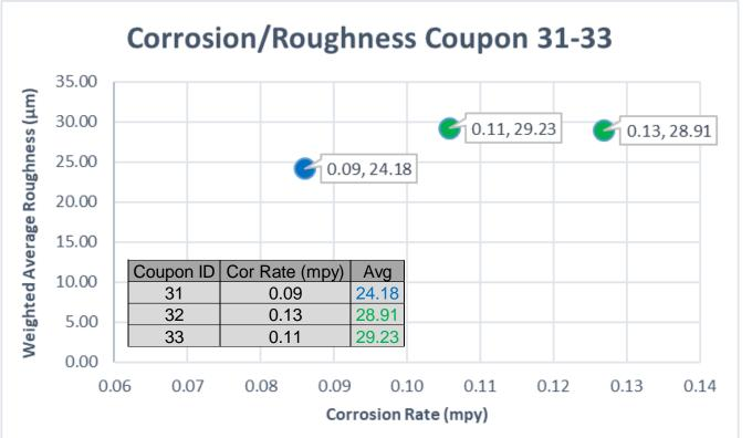
In the graph above the weighted average roughness was calculated by the percent surface area of the side (Ra #) divided by the total surface area then multiplied by the side surface roughness.
