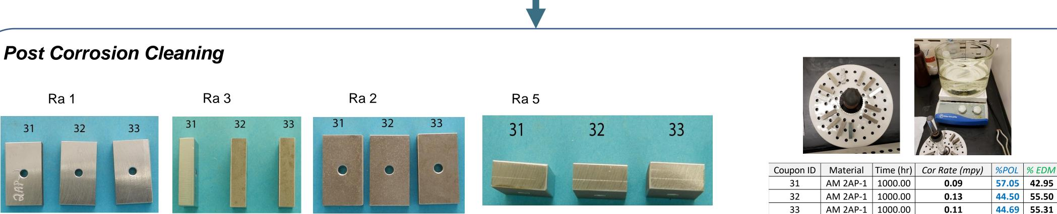
• The corrosion weight loss stabilized four cleaning cycles, each cycle was 8 minutes with predetermined temperature and flow requirements based on ASTM-G-31.
