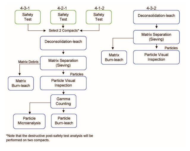
Figure 1. Proposed safety testing and analysis work flow on four PBMR Compacts (note that Gamma counting has been deleted for Compact 4-3-2.
