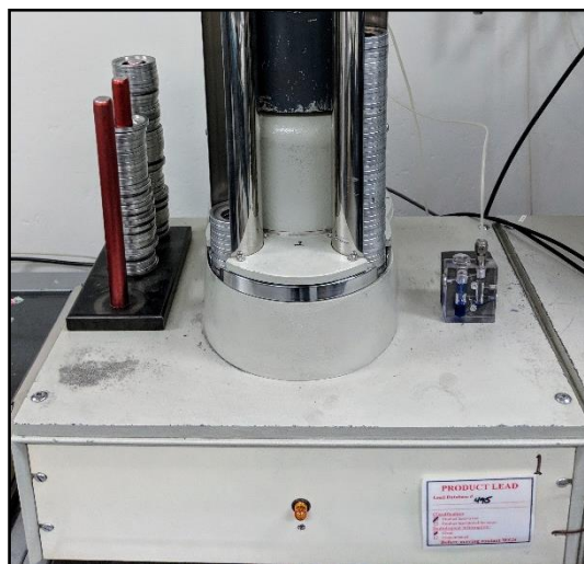
FIG. 1. The 4-channel counting system utilizes original sample-changing hardware and proportional gas detectors to measure the gross beta-particle activity of irradiated fission wires [1].
