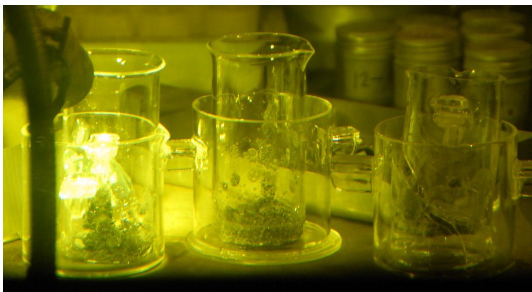
Figure 6. Capsules 3, 6, and 5 graphite holders after oxidation. Tall-form beakers were put inside overburden containers after chemical reactions with the quartz tall-form beakers started.
