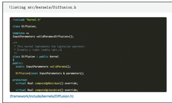
Fig. 5. Example use of the “listing” command within (upper) markdown file that results in (lower) a rendered copy of source code.
