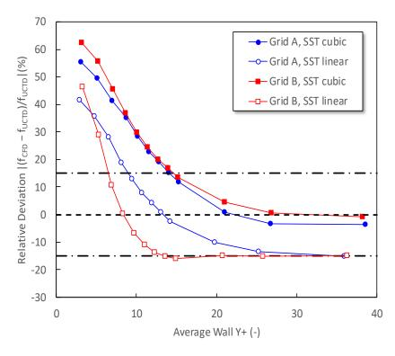
Evaluation of the Friction Factor Correlations and CFD Result for the SFR 217-pin Wire-wrapped Fuel Rod Bundle (Error bar:  $\pm$ 20% of UCTD).
