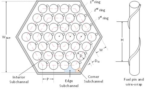
The present work aims at evaluating the existing friction factor correlations for 217 pin wire-wrapped fuel rod bundle of SFR and the range of applicability of the correlations to identify the preferred correlation for the SFR analysis.
