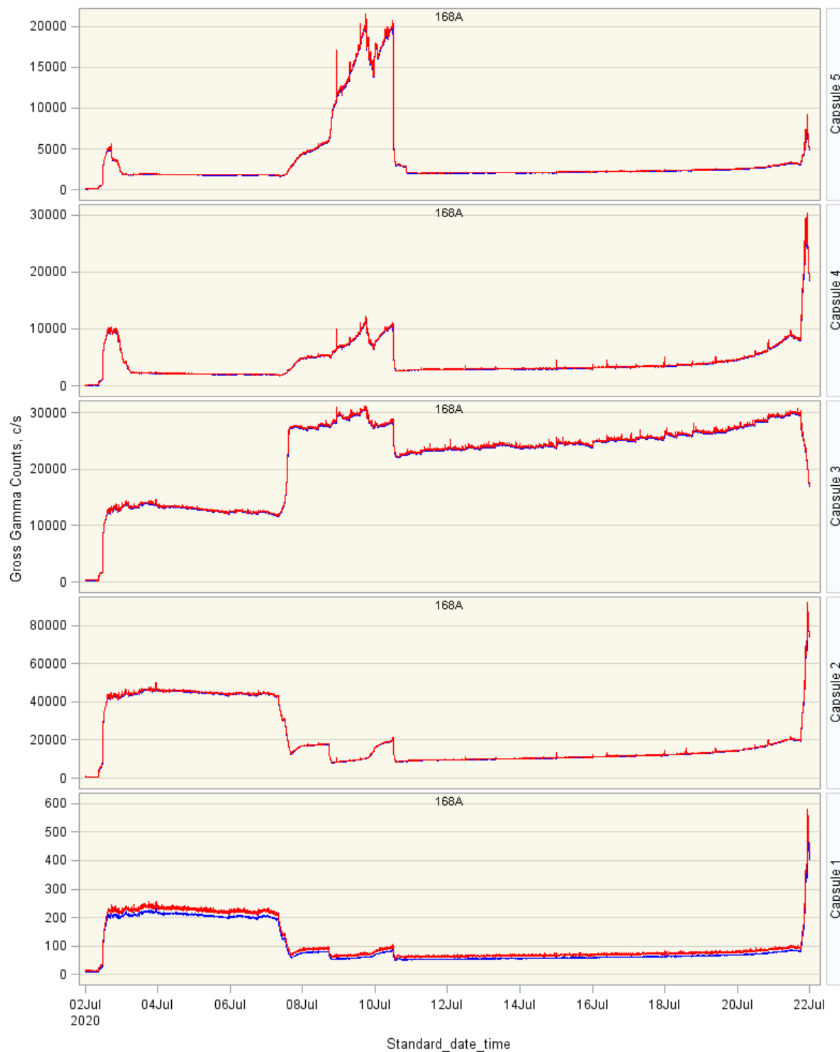
Figure 23. Typical spikes associating with particle failures are observable in Capsules 2 and 3 based on 5-minute peak and average GG counts between July 2 - 22, 2020 during 168A.
