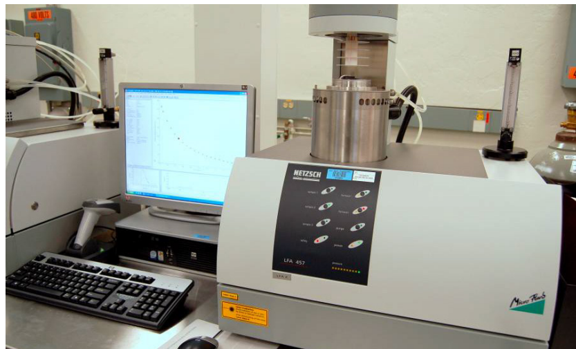
Figure 15. Laser flash apparatus measurement station for determination of thermal diffusivity.
