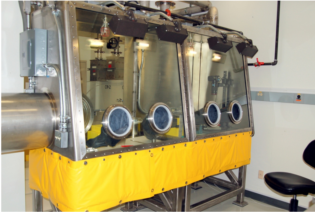
Figure 1. The CCL glovebox used to visually inspect graphite samples, perform initial dimensional measurement, and repackage samples for storage in the irradiated graphite vault in Laboratory C-19.
