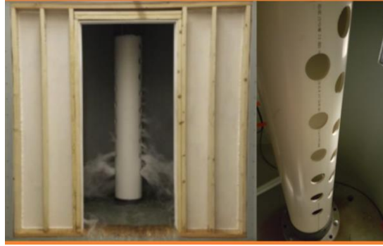
Figure 5-11 ISU Flood Testing Facility Pump System 1 - Inlet [34]
