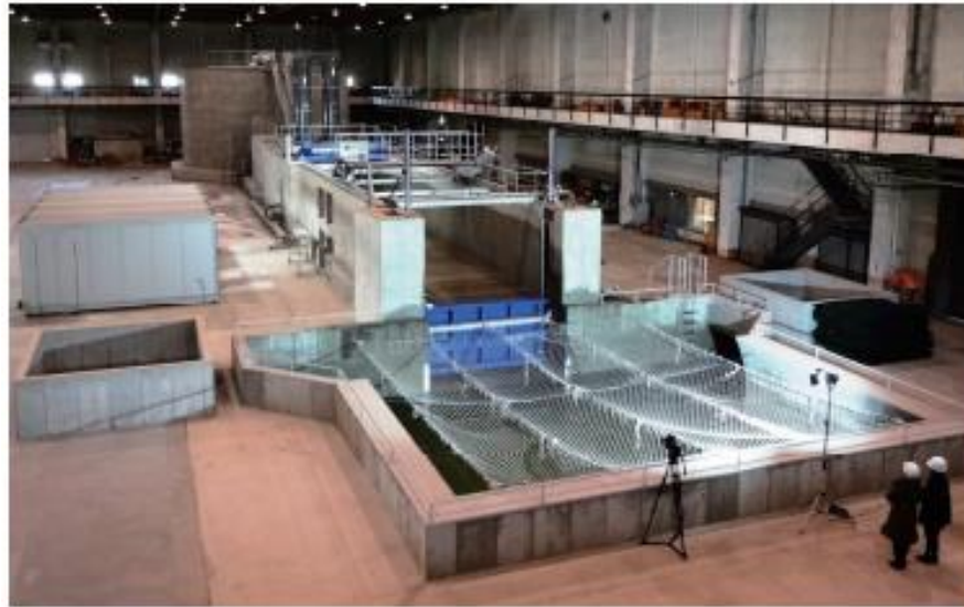
Figure 5-29 Japan CRIEPI Large-Scale Tsunami Physical Simulator [62]
