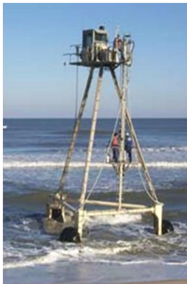
Figure 5-25 USACE ERDC CHL CRAB Vessel [54]
