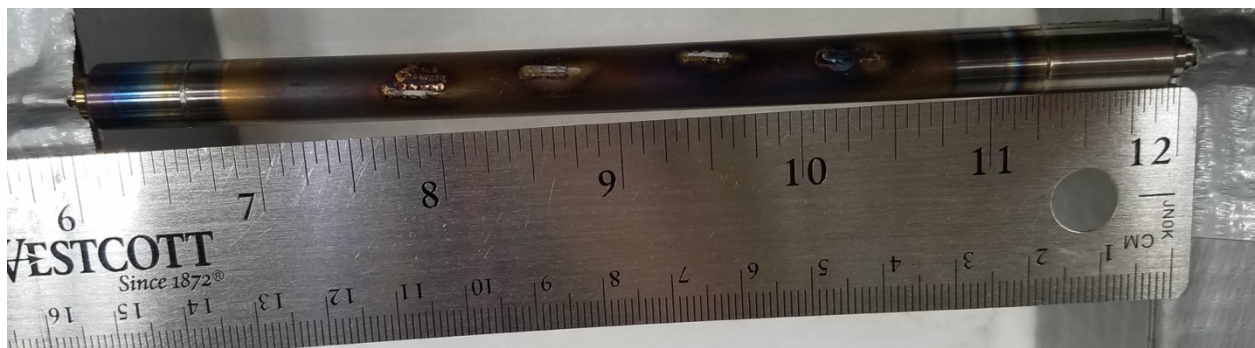
Figure 13. Post-transient visual examination of SETH-G rodlet.
