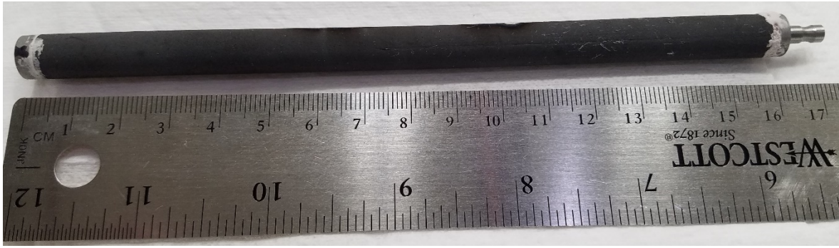
Figure 14. Post-transient visual examination of SETH-H rodlet.
