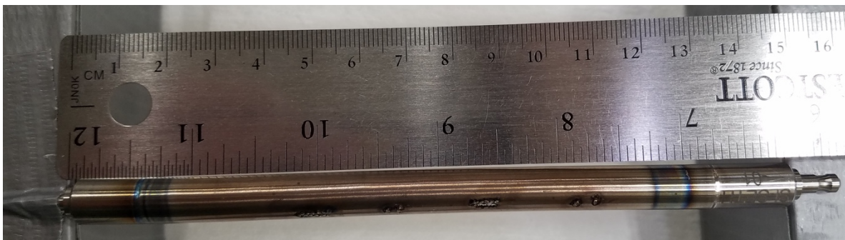
Figure 12. Post-transient visual examination of SETH-F rodlet.
