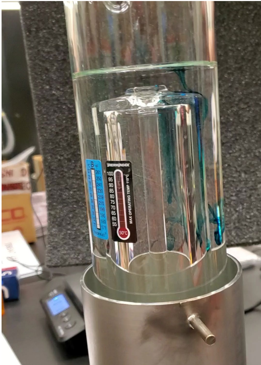
Figure C- 11. Dye addition for the liquid mixing test.
