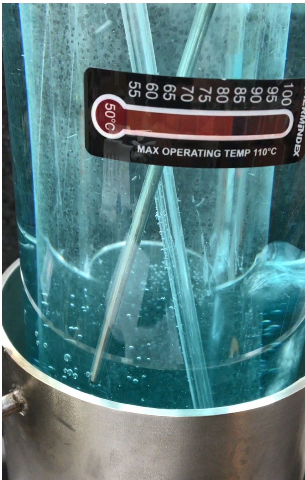
Figure C - 7. Sparge (front) and TC positions during heating test.
