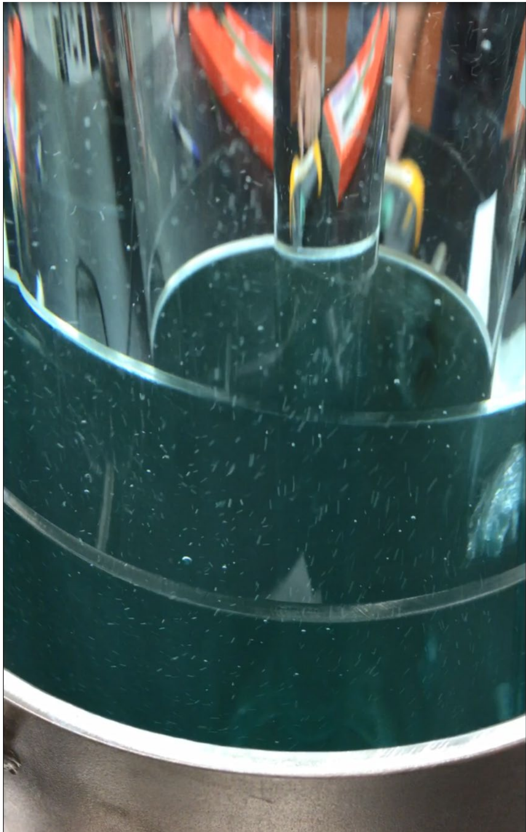
Figure C - 6. Sparge (right side of image) in annulus and small bubbles showing water circulation patterns.
