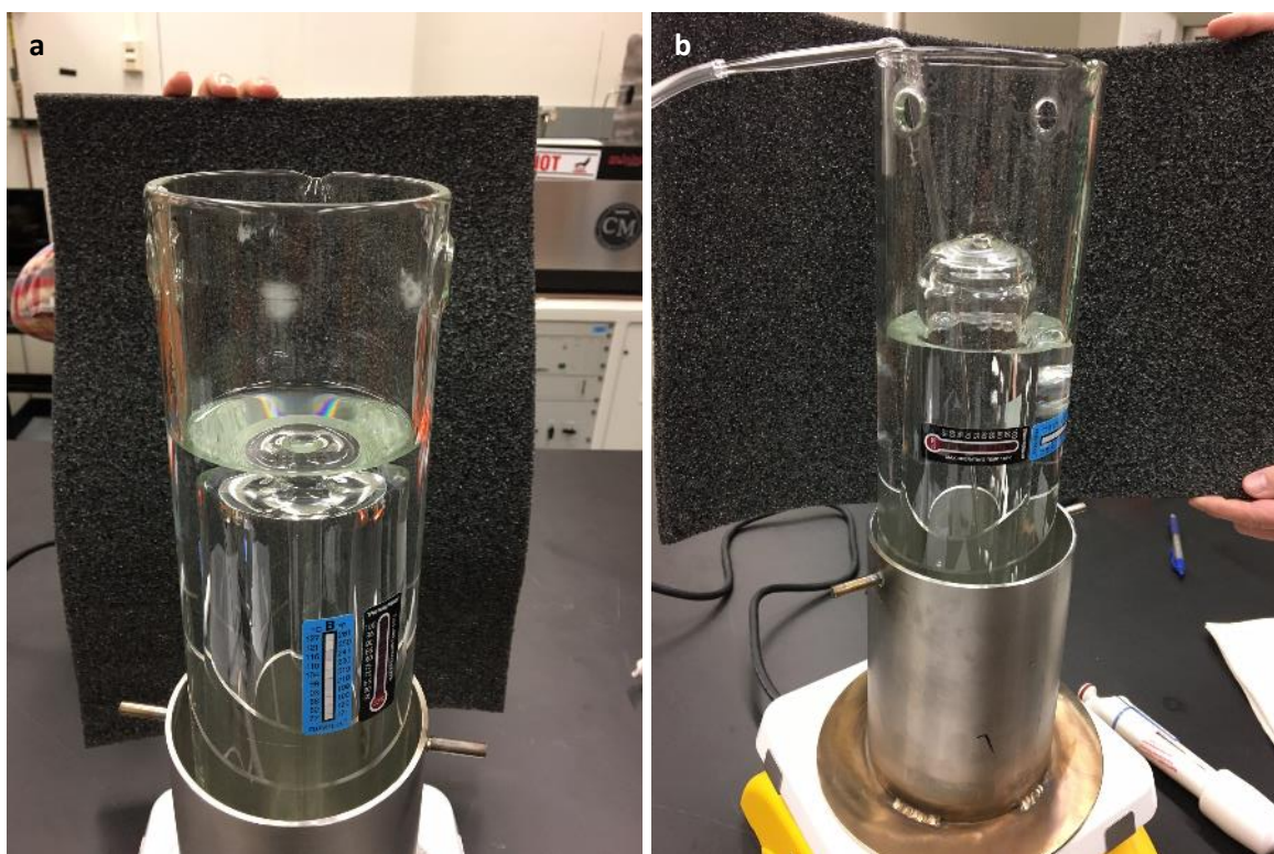
Figure C - 4. First (a) and second (b) glass leach vessels in base and on hotplate.
