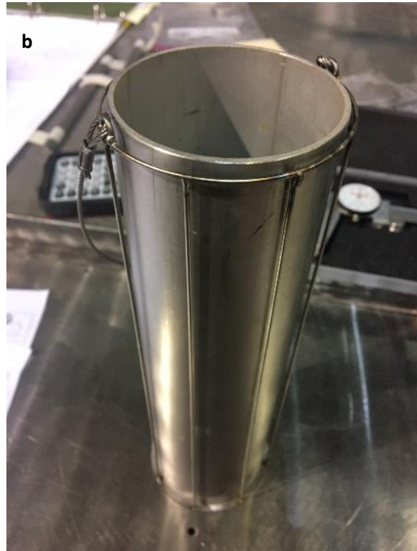
Figure C - 3. Test fit of simulated capsule shell in prototype basket (a) and actual basket at American Fabrication (b).
