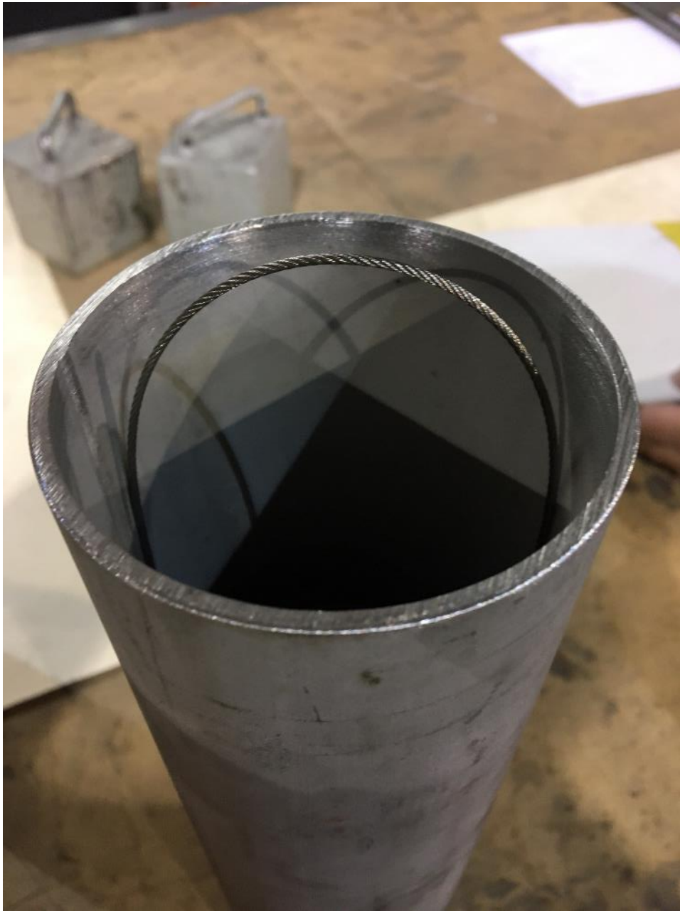
Figure C - 9. Capsule shell basket fully inserted between nested 3" Sched. 10 and 1.5" pipes.
