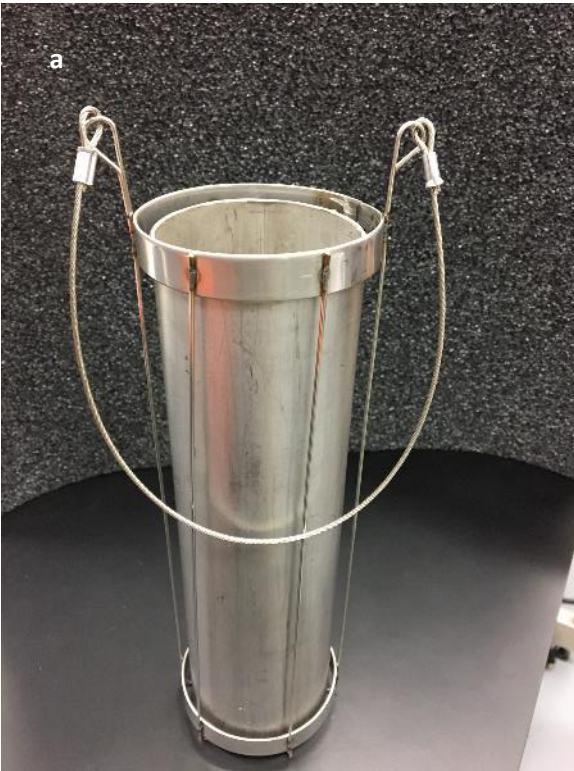
Figure C - 3. Test fit of simulated capsule shell in prototype basket (a) and actual basket at American Fabrication (b).
