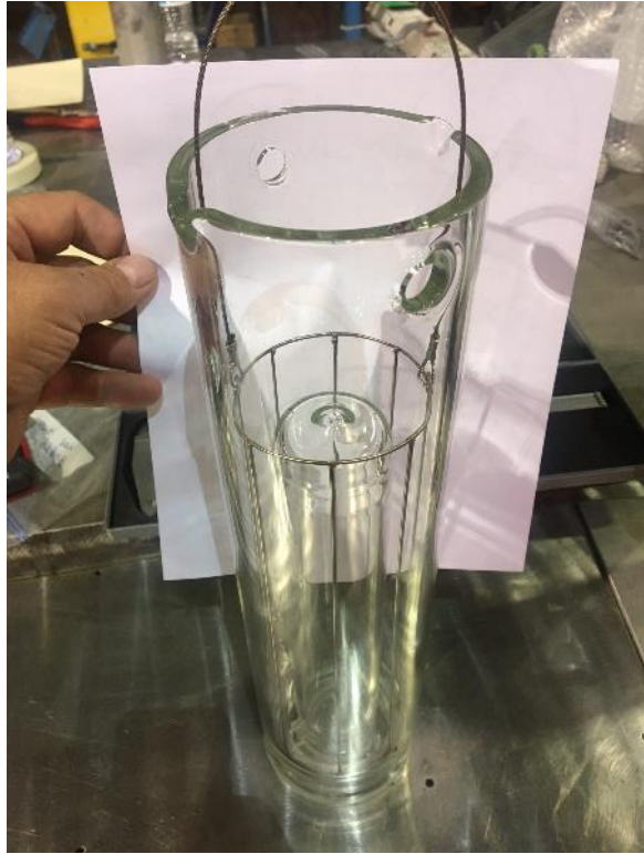
Figure C - 2. Test fit of capsule shell basket into glass leach vessel at American Fabrication (basket fabricators).
