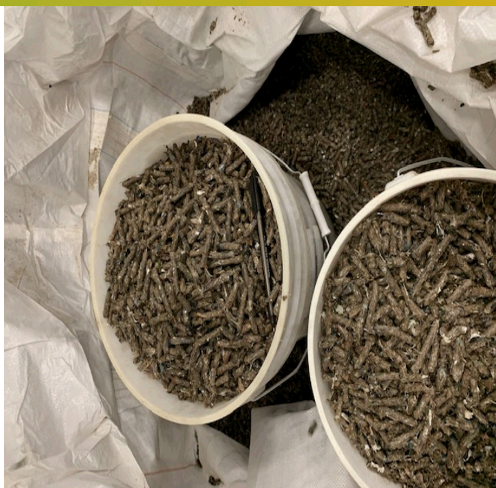
MSW pellets made at about 25 % (w.b.) moisture content using 1/2 - inch hammer mill grind.
