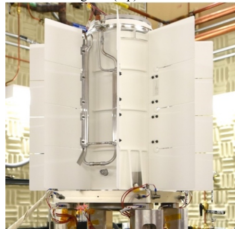
Fig. 4. MMRTG mounted on the vibration test fixture.
