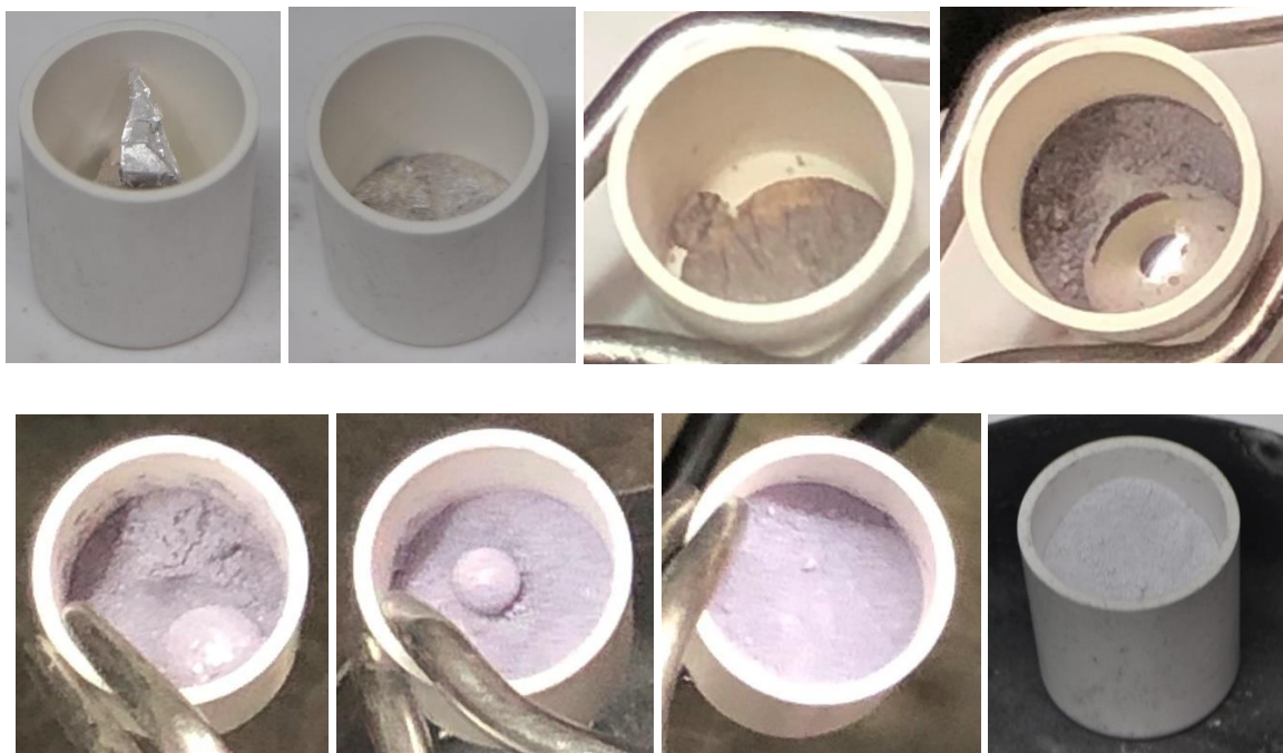
Fig.1. Progression of sodium metal deactivation for run 1 from left to right, top to bottom.
