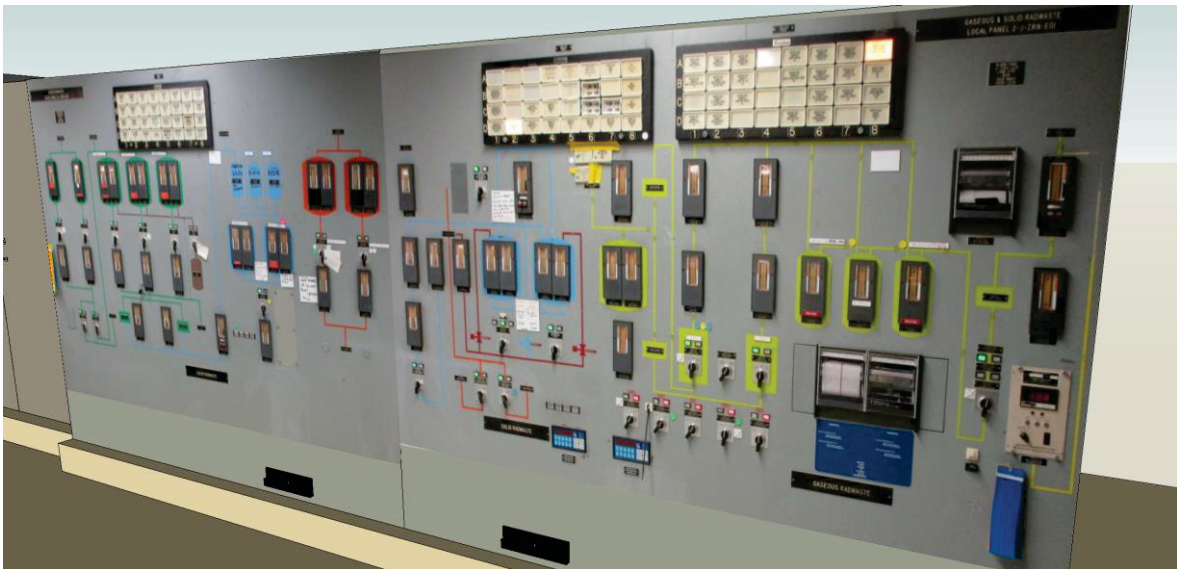
Figure 24. 3-D model of the LRS panel and gaseous and solid radiological waste panel in existing radiological waste control room.
