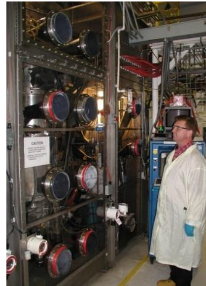
Industrial Scale 150-mm Coater (BWXT)
