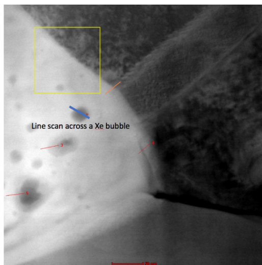
Figure 11. EDS line scan (short blue line) showing xenon in a gas bubble.
