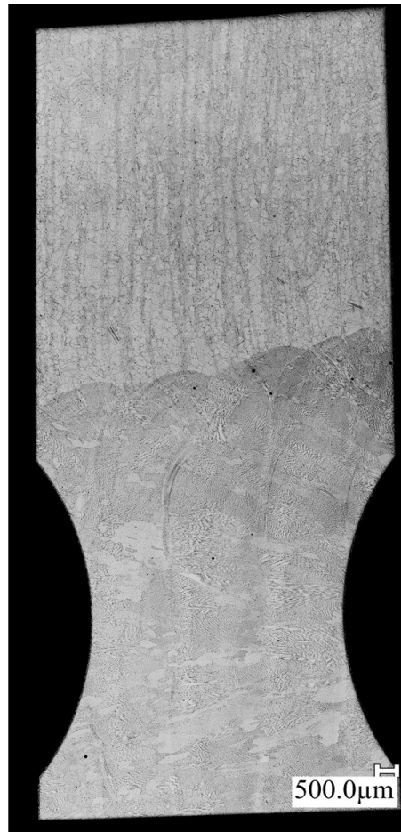
Figure 23. Etched cross section of the weld metal large-radius U-notch interrupted creep test performed at 800°C, 80 MPa to 800 hours.
