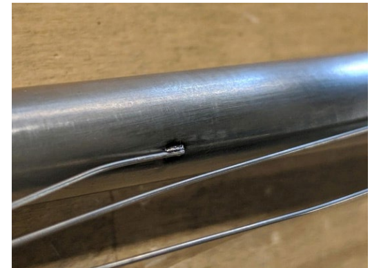
Thermocouple weld mockup
