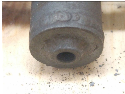
Thermowell (0.125" ID) in sodium filled heat pipe (0.625" OD) for distributed temperature sensor deployment
