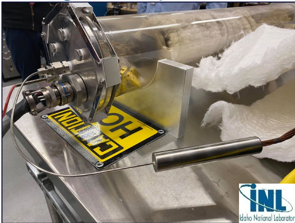
Thermocouple installed in SPHERE
