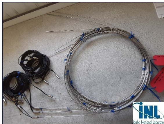
SPNDs to be thermally tested in MAGNET
