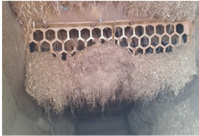
Plugging of Grinder Screen
