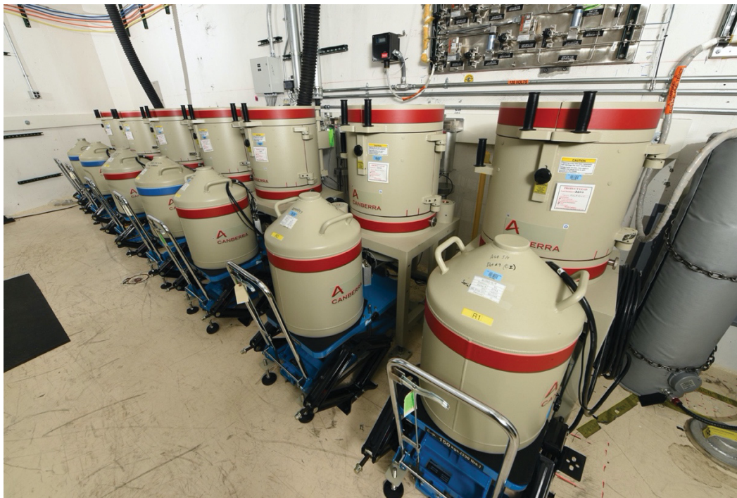
Figure 3. The FPMS in ATR-670, 1A primary. Each of the five AGR-5/6/7 Capsules has a corresponding FPMS. This system also contained two on-line spares.
