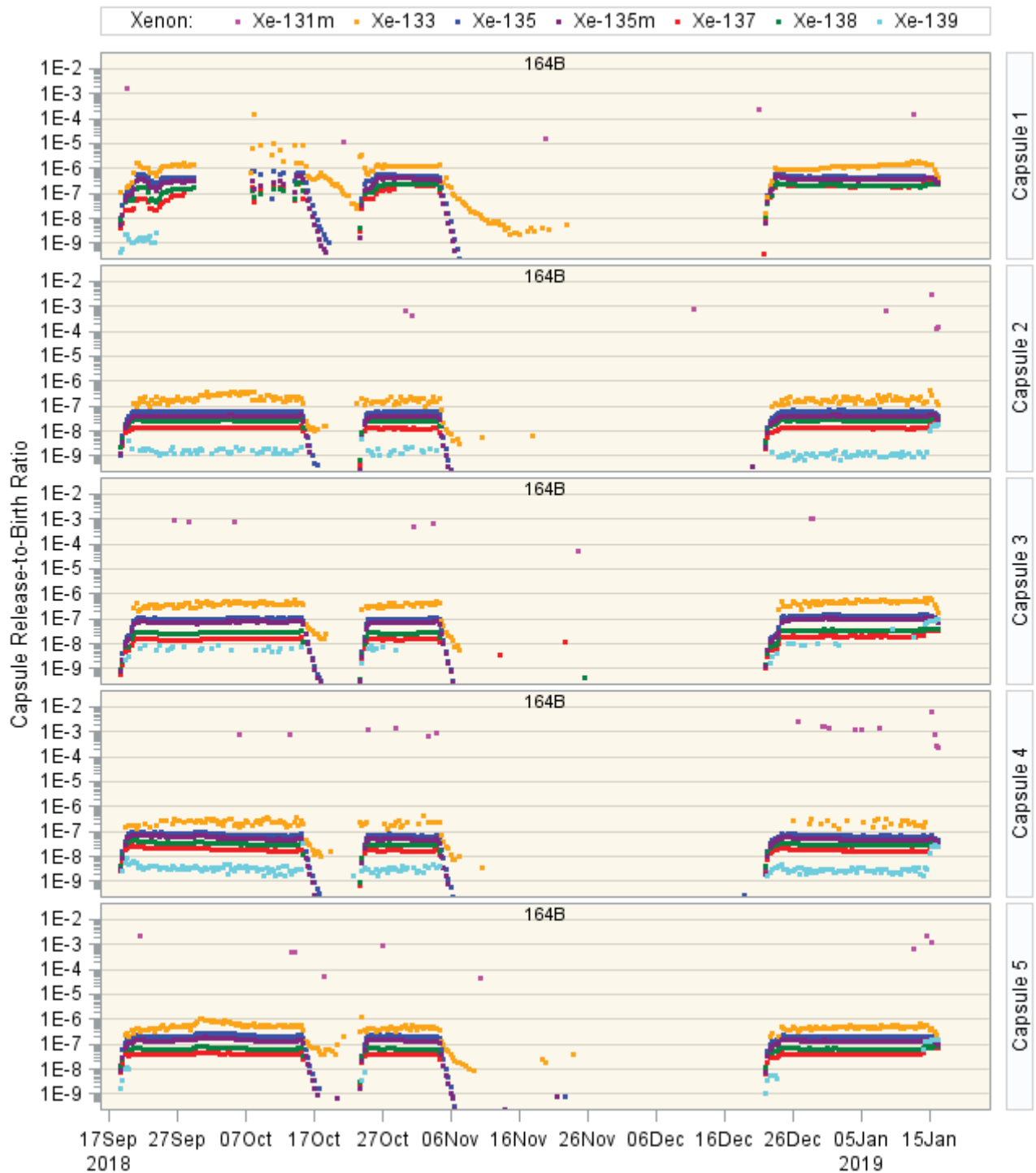
Figure 18. Cycle 164B release-to-birth ratios for selected xenon isotopes for AGR-5/6/7 Capsules 1–5. The trailing Xe-133 in this figure is from isotopic decay. The half-life for Xe-133 is 5.24 days.
