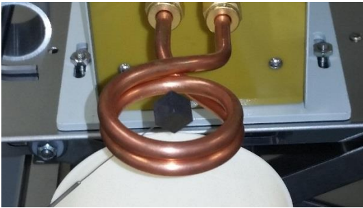
Figure 3. Test of TREAT DAS by heating a small graphite block with an embedded TC.
