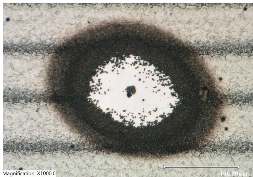
Figure 5. Removal of the printed sensor region in the center of a spot irradiated with laser pulses with energy of 4\text{ }\mu\text{J} .
