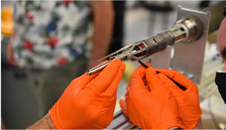
Insertion of rodlet/TC assembly into holder
