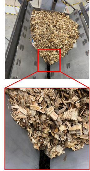
Figure 1: (a) A biomass material Process Development Unit at Idaho National Laboratory, Idaho Falls, ID, USA. Hoppers are marked out in the yellow boxes. (b) An example of woody biomass material arching in a wedge-shaped hopper.
