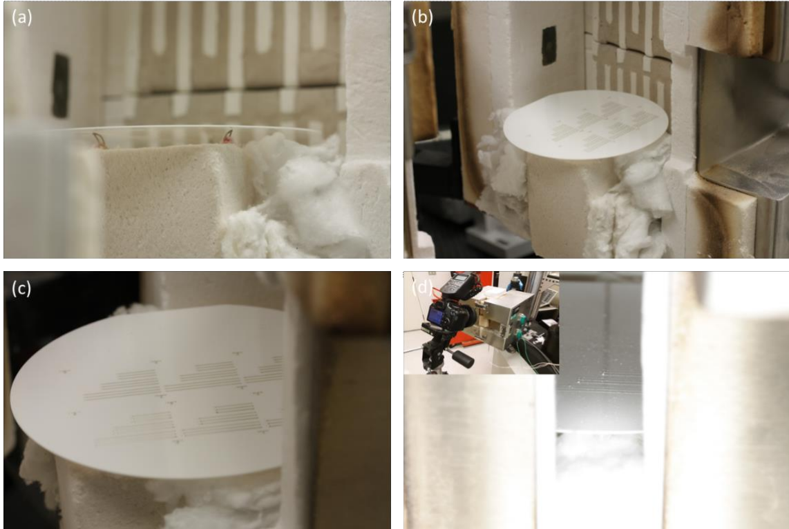
Figure 4– Experimental Set-Up: (a) two thermocouples positioned under the alumina substrate, (b) printed silver melt wire array on alumina substrate, (c) magnified image of the substrate positioned inside the furnace, and (d) magnified image of printed silver melt wire lines on alumina substrate.
