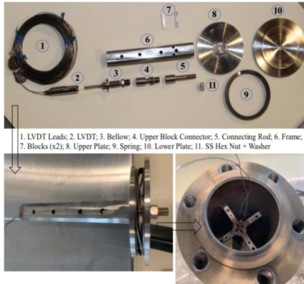
Figure 10 – Autoclave testing using calibration fixture.
