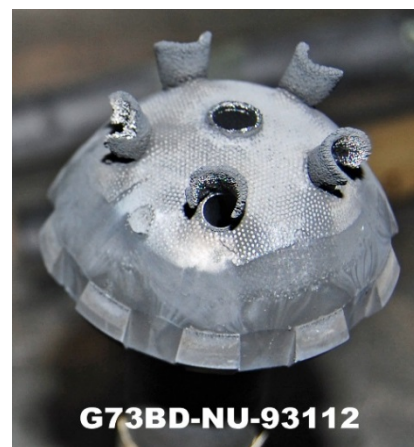
Figure 10. Former gas-distributor nozzle with a dimple pattern in the SiC accretions.
