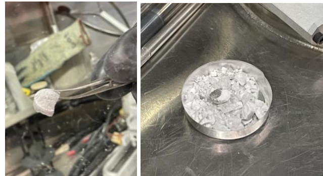
Fig. 5. Extracted salt following prototype testing.
