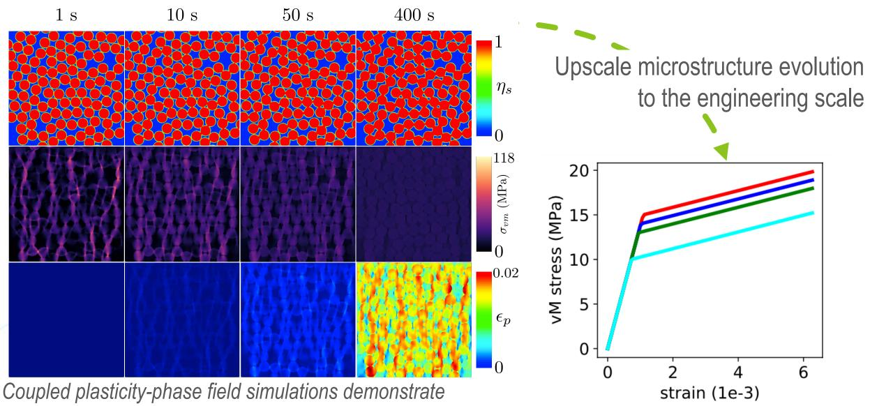
Coupled plasticity-phase field simulations demonstrate the key role of stress in driving diffusion processes in sintering. Top row: microstructure, middle: effective stress, bottom: effective plastic strain.
