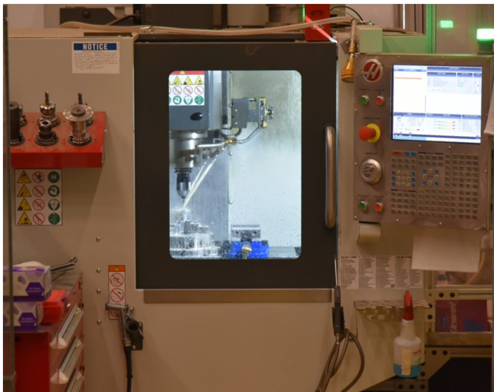
Figure 3. A \text{UO}_2 pellet is fixtured within the HAAS Mini-Mill for drilling.
