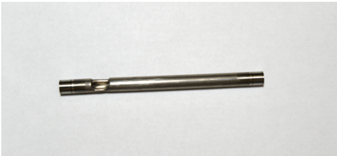
Figure 5. Rodlet exhibiting complete collapse of the cladding within the plenum region after HIP run.
