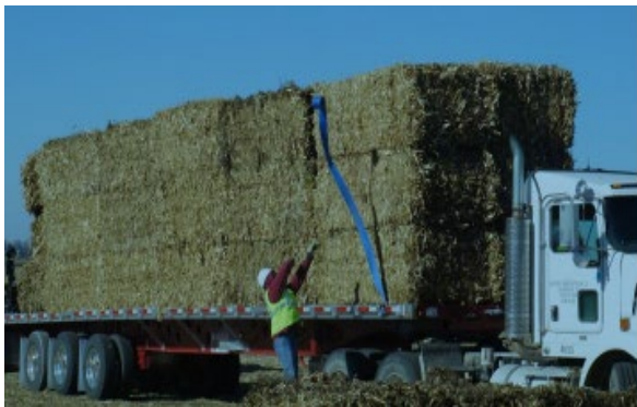
(a) Manual bale securing system
