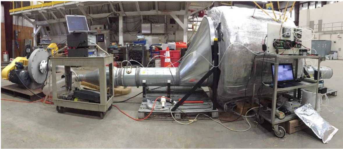
Figure A-3. Bale dryer/bale permeameter fabricated and used by INL to measure drying, internal temperatures, and moisture loss in whole bales. Air flow is from the right to the left in the photograph. The instrumentation on the right records the temperature and relative humidity of the air entering and exiting the bale, the internal bale temperatures, and the pressure drop across the bale. The instruments on the left periodically sample the inlet and outlet gases and measure CO 2 , water vapor, and gas tracer (SF 6 ), which is metered in from the silver bag at bottom right.
