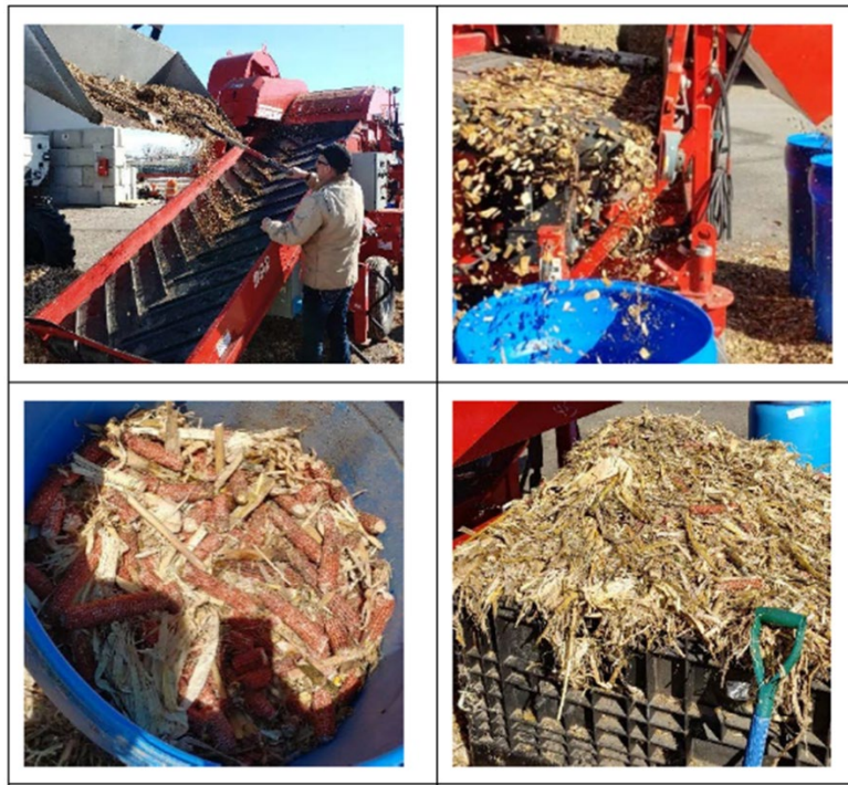
Figure 3. Spudnik air classifier for corn stover anatomical fraction separation.
