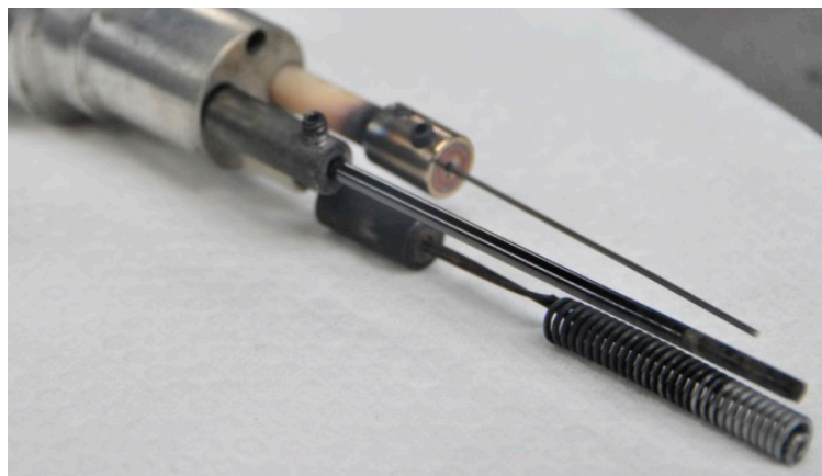
Figure 2. Three-electrode set up (iridium wire as the working electrode; glassy carbon as the pseudo reference electrode and molybdenum coil as the counter electrode).
