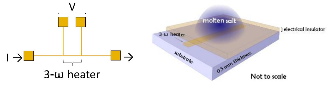
The magnitude of the temperature rise of the resistor,  $\Delta T$ , will depend on the thermal conductivity of the surrounding material. The temperature change results in a resistance, R, and voltage fluctuation across the resistor. Subsequently, by measuring the resultant voltage drop, V, at the first ( $\omega$ ) and third ( $3\omega$ ) harmonics, the temperature oscillation can be determined. The 3-omega voltage,  $V_{3\omega}$ , is proportional to the temperature oscillation.
