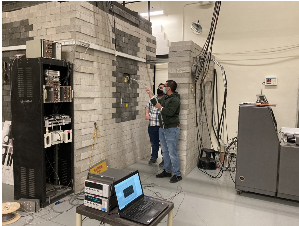
Installing SPNDs in AGN-201 Rx
