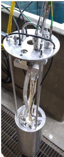
Figure 1: Heated irradiation furnace rig.
