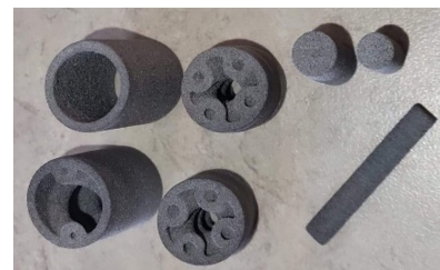
In partnership with Advance Cooling Technologies Inc., INL produced porous metal materials for use in heat pipes.
