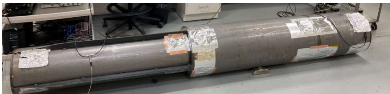
Figure 5. Canister with RF and acoustic transmitter (right side) and receiver inserted (left side).
