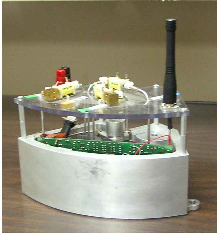
Figure 1. The initial integrated sensor system prototype was fabricated in 2000 and designed to measure hydrogen, relative humidity, and temperature in a CPP-603 storage canister
