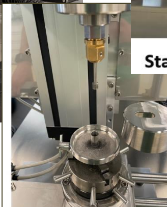
Top pellet removed and oxidation cleaned from inner and outer surfaces of the cladding
