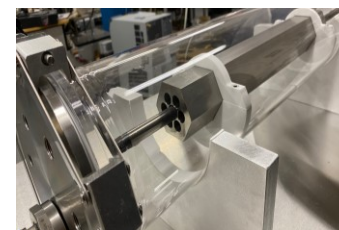
Quartz tube allows testing in vacuum or inert gas environments
