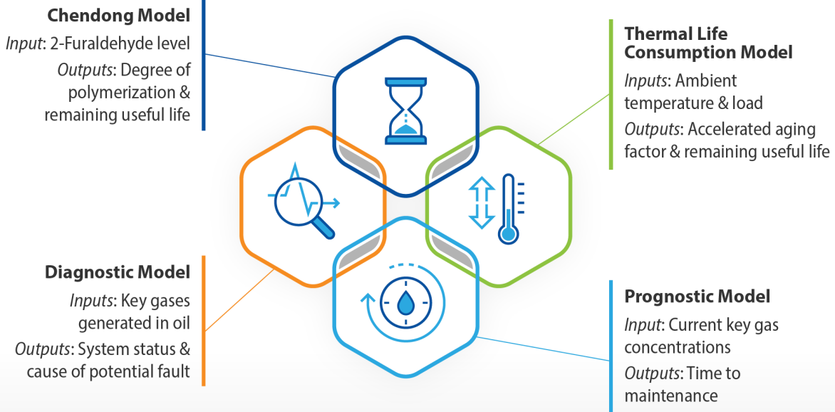
Figure 1. These four models synergize with regard to transformer health monitoring by incorporating different inputs to produce actionable outputs.
