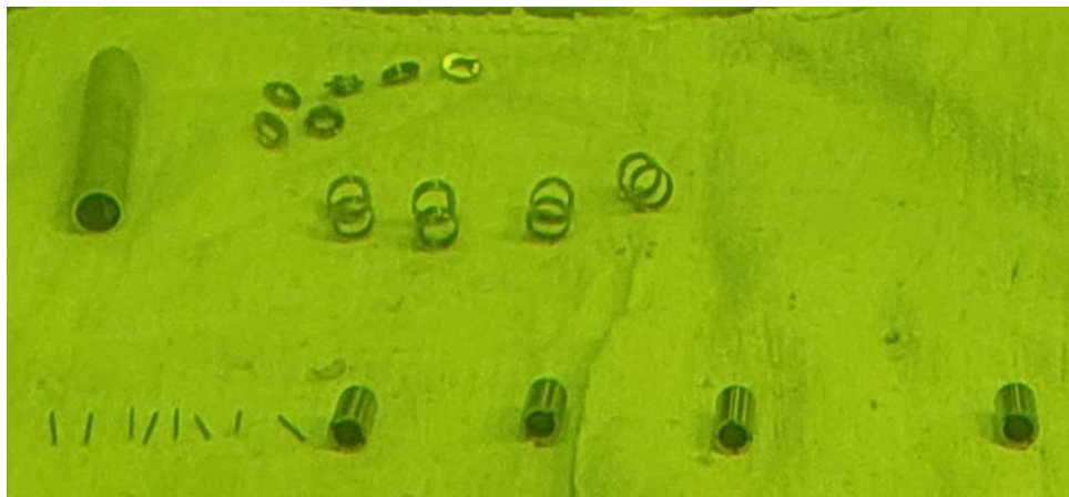
Figure 3. Axial tensile test cladding specimens being sorted and identified during capsule disassembly in the ORNL 3025e hot cell facility.
