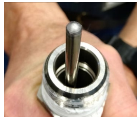
Figure 4. Fuel pin drilled, pressurized and rewelded for THOR-C-2
