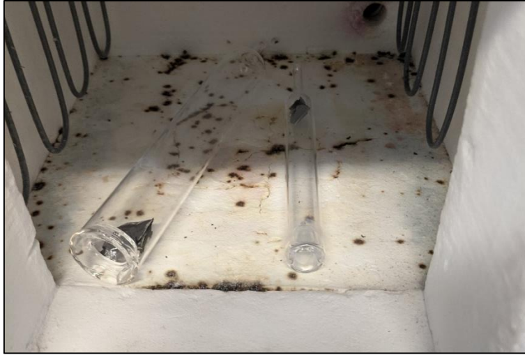
Figure 4. Heat-treatment samples wrapped in foil, sealed in quartz ampoules, and placed inside furnace.
