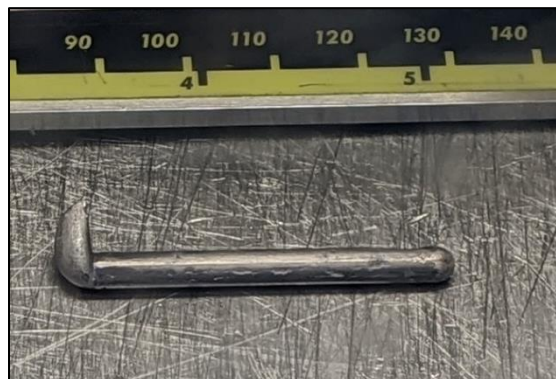
Figure 2. 4 mm diameter pin of U-Nb-Zr.
