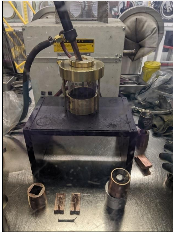
Figure 1. Arc-melter with button and split hearths.
