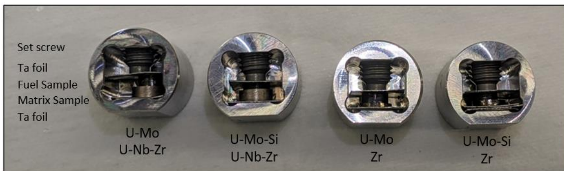
Figure 5. Stack up of diffusion couple assemblies for interaction testing.
