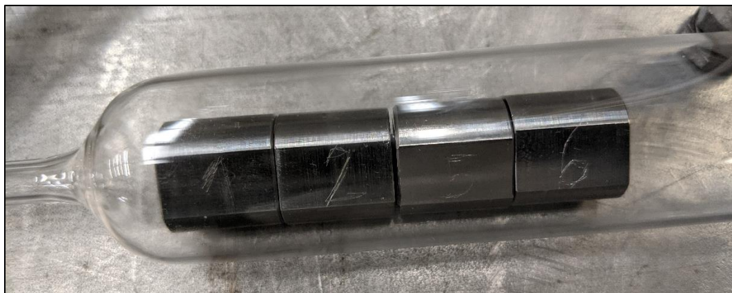
Figure 7. Diffusion couple assemblies sealed in quartz ampoule under high vacuum.
