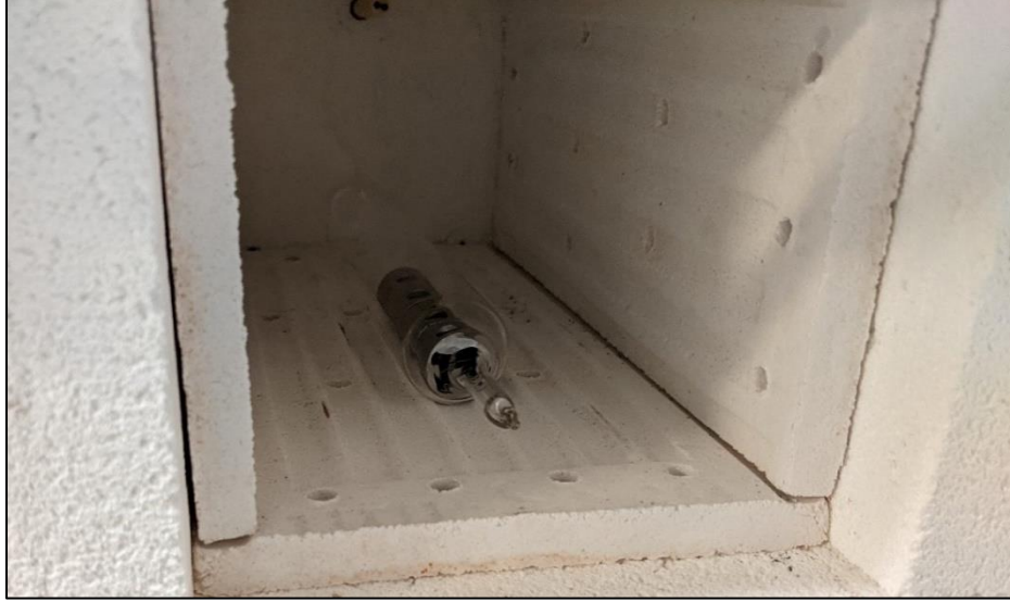
Figure 8. Diffusion couple assemblies sealed in quartz ampoule under high vacuum.
