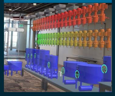
Displaying real temperature values recorded by physical instruments on a 3D model using mixed reality
