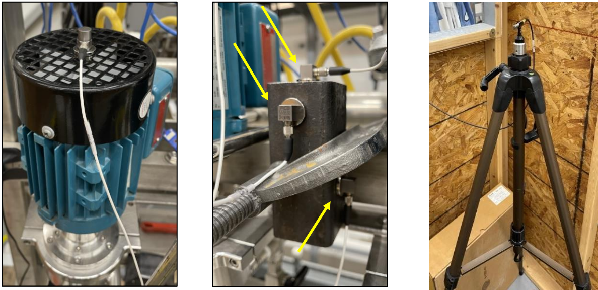
Figure 3. The image on the left shows an accelerometer axial to the contactor motor. The image in the center shows directional accelerometers deployed on contactor framework. The image on the right shows a microphone used to record operational sounds emitted from the contactor system.
